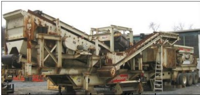
Older equipment may be as efficient as new, but may not meet noise emission requirements
